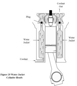
Thus, all heat engines need cooling to operate. Cooling is also needed because high temperatures damage engine materials and lubricants. Internalcombustion engines burn fuel hotter than the melting temperature of engine materials, and hot enough to set fire to lubricants. Engine cooling removes energy fast enough to keep temperatures low so the engine can survive.
